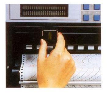
The ink cartridge and chart paper can easily be replaced without removing the internal unit of the recorder.
